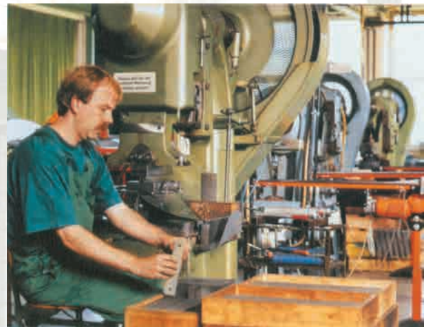
Fig.7: Production of core laminations
