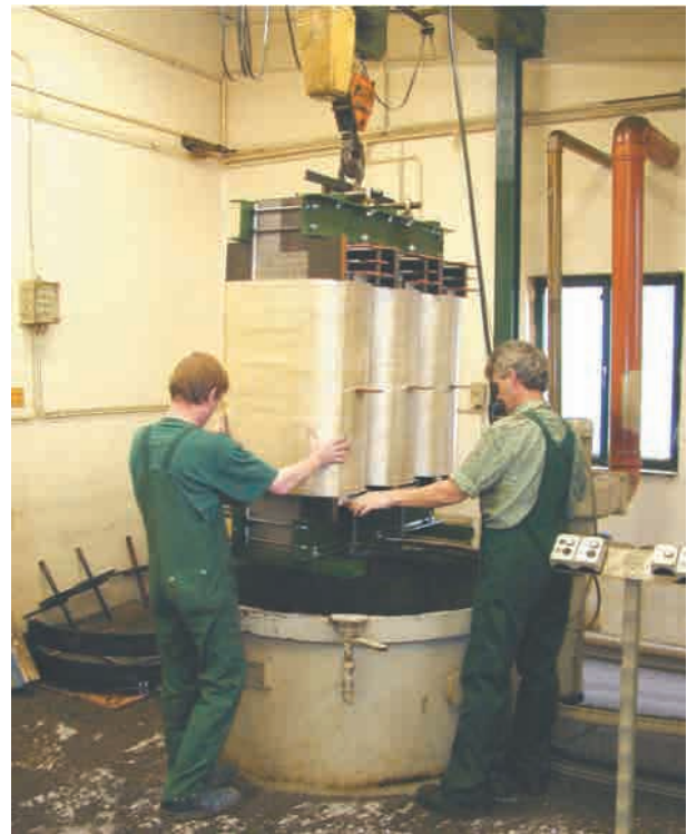
Fig.9: Vacuum/overpressure impregnation equipment
