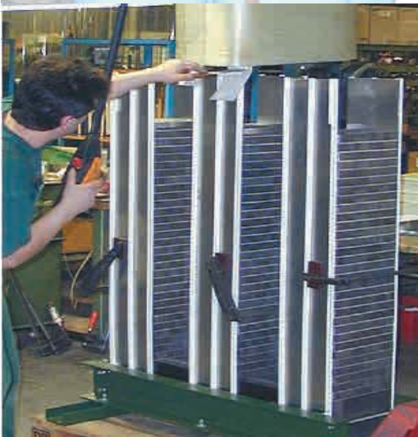
Fig.4: Assembly of a three phase iron cored reactor
