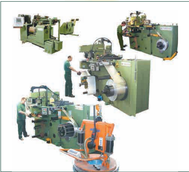
Fig.8: Computer controlled winding machines
